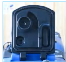
污水箱内水满保护装置 Sewage tanks with full water device
